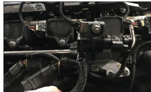
Remove the vacuum line from the sensor.
